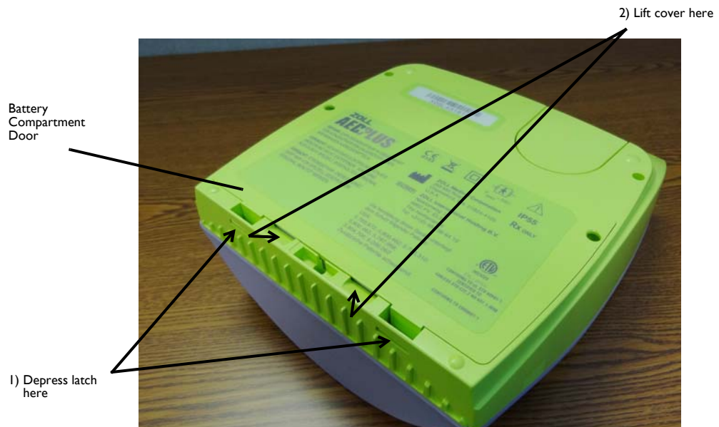
Figure 7: Removing the Battery Compartment Door
